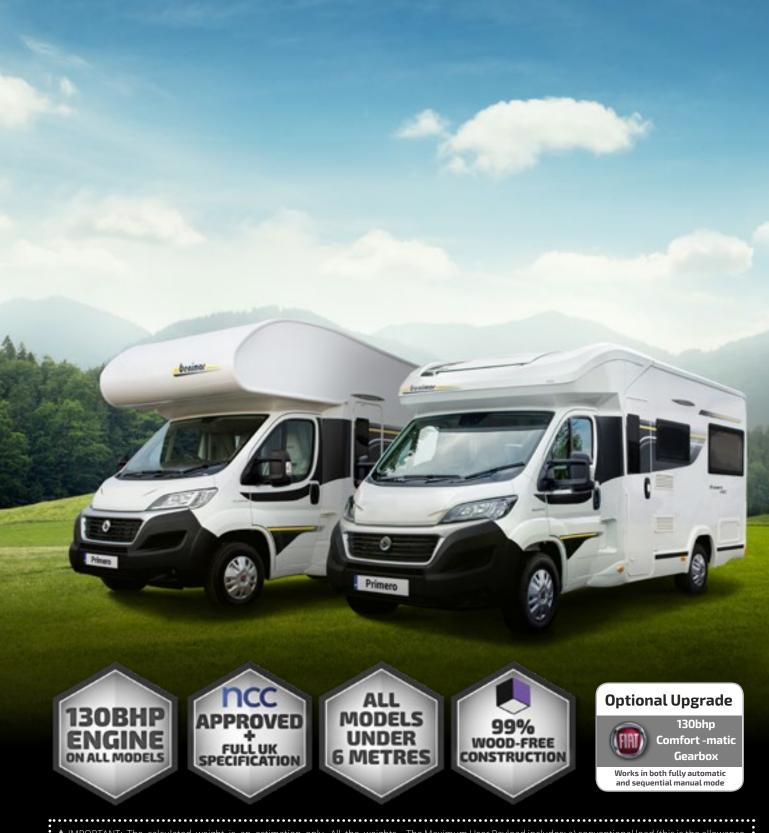
† IMPORTANT: The calculated weight is an estimation only. All the weights mentioned in this catalogue are according to the European Directive 1230/2012 and to the EN 1646-2 standard. The calculation of the weight includes; 90% of fuel in the tank, 1 gas bottle, 50 litre fresh water, 1 person to drive (75 kg), 10 kg luggage. All masses and weights are subject to a tolerance of +/-5% complying with the European Directive 1230/2012.
