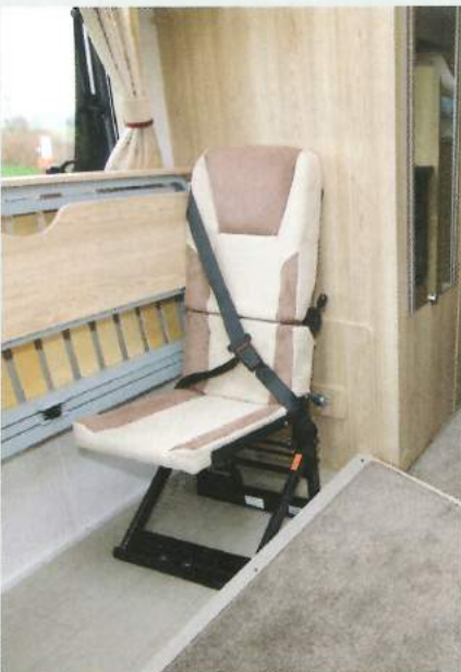
These fold-away Aguti travel seats have steel frames and three-point seatbelts
