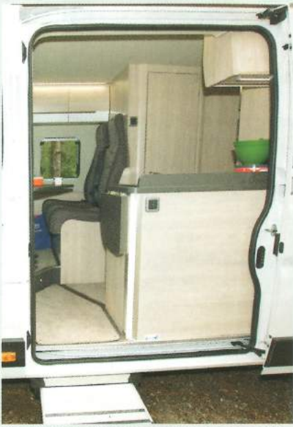
The kitchen stretches part-way across the door, which has an electric step
