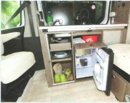
There's good storage in the galley and a small, front-loading compressor fridge
