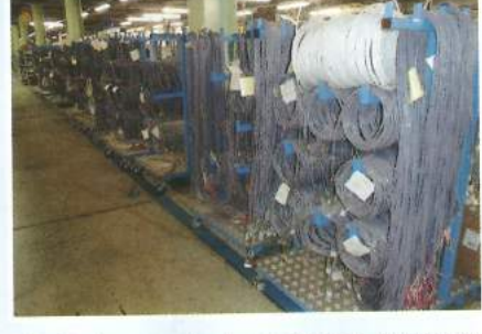
12 As space is always limited, hundreds of cables they have to be created and delivered on a 'just-in-time' basis, so that they're ready and waiting when the correct model is being built.
