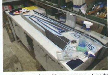
18 The vinyl graphics are prepared ready for applying. These are designed by an in-house art team using the latest on-trend colours and styles. They're made in tough, weather-resistant vinyl on site. >>
