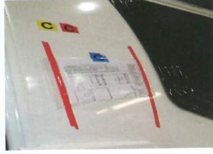
17 All the way along the production line, the build is carefully logged, including the specification and its quality-control status. Any issues are noted, to be addressed before the tourer is completed.
