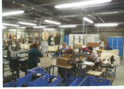
11 Caravelair's wiring looms are made in-house. Each one's created to fit a specific caravan, sometimes with bespoke options. This work requires extreme focus and precision. It's no place for a man then!
