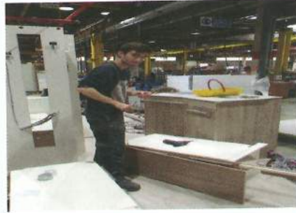
5 Meanwhile, the caravan's cabinetry is being prepared and checked ready for fitting, in a different part of the factory. Once fitted, these fixtures will add further rigidity to the body panels.
