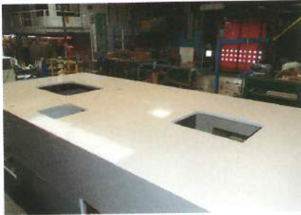
10 The edges are sealed with mouldings. Now it just needs its rooflights to be fitted. In the rooflight apertures, you can see how rigid insulating foam is sandwiched between thin-but-strong layers of GRP.
