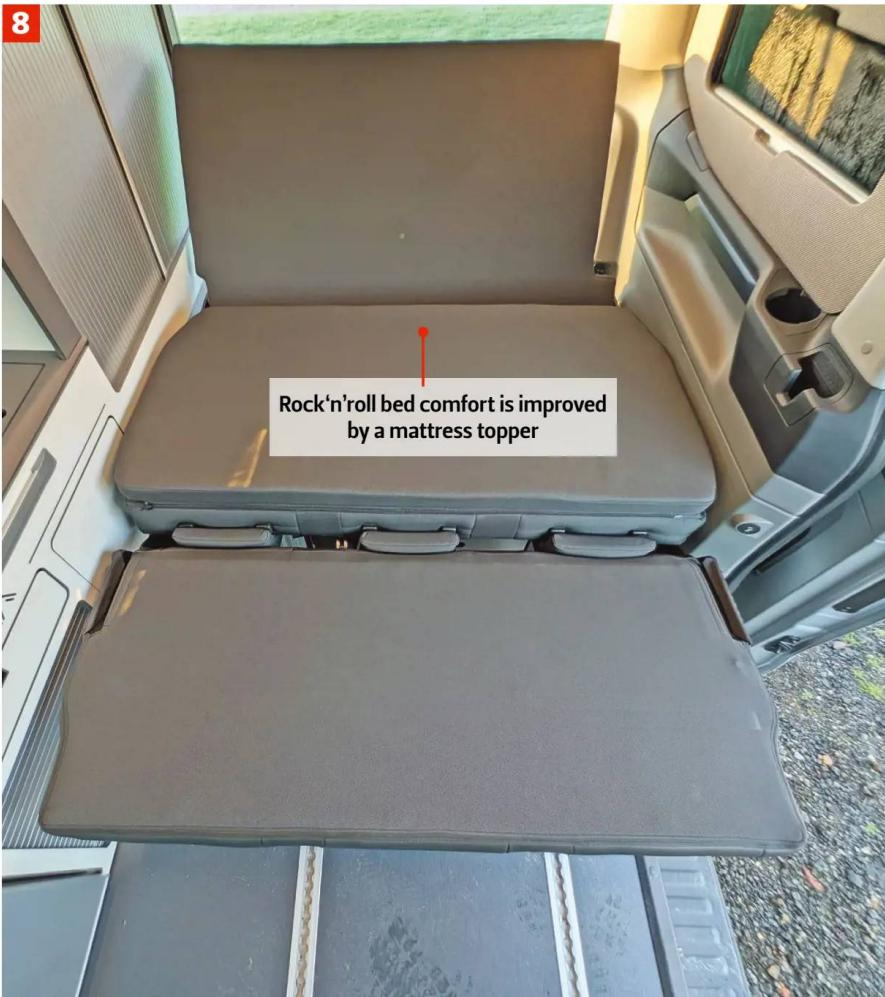
Although there are five travel seats (with two ISOFIX points), the Panama offers four berths for sleeping. The bench seat uses the sliding floor track system to become an 1890 x 1140mm rock'n'roll bed (8). You aren't expected just to lie on the folded down seats, because a mattress topper folds over to provide a very smooth and comfortable surface.
