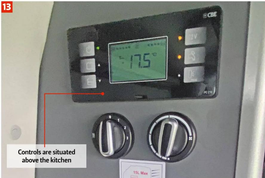
Water and power is controlled and monitored via a digital panel above the kitchen, accompanied by two dials that control the heating (13). Since this is a gas-free model, the heating is a 1000W electric heater. One tester tried the 'van during a warm September, so didn't need to use it, but another found that in late November the 'van took around an hour to warm up fully.
